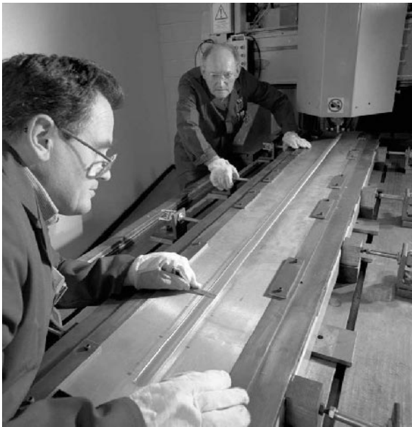
8.15 2 metre long friction stir weld in 10mm thick A6082 alloy. Courtesy of TWI Ltd.
