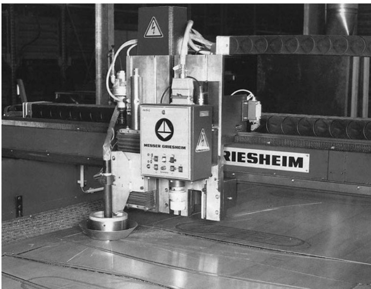
4.1 Fully programmable CNC plasma-jet cutting system. Courtesy of Messer Griesheim.
