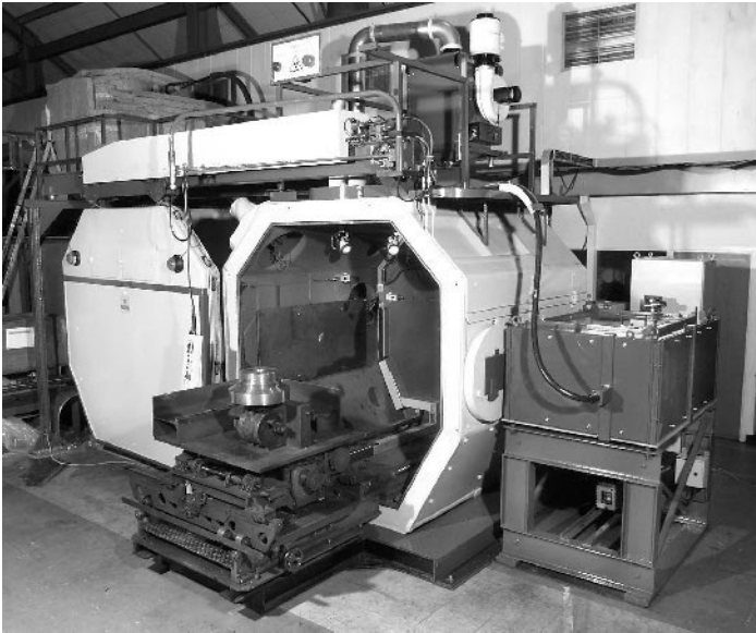
8.8 A 2 m 3 chamber, 100 kW, electron beam welding machine, showing the open vacuum chamber. It is capable of welding up to 200 mm thick aluminium. Courtesy of TWI Ltd.
