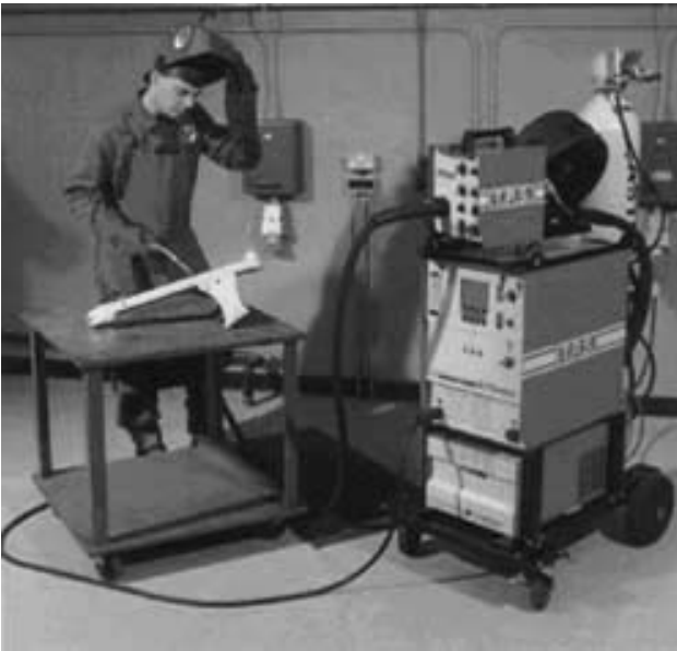
7.2 Illustrating the general arrangement of the power source, wire feeder gas cylinder and work area. Courtesy of TWI Ltd.
