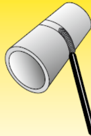
Pipe fixed with axis horizontal, welding downwards: PJ/5G
