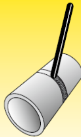
Pipe fixed with axis horizontal, welding upwards: PH/5G
